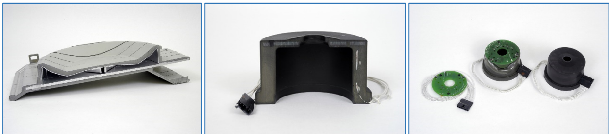
Figure 1A 1/4" aluminum plate and a steel alloy strap are molded into a single part, as shown above. Encapsulation using RIM was chosen for two different applications on one product manufactured by Kendro Laboratory Products. Above (right), sophisticated electronics are encapsulated to protect against damage.
