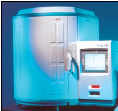
When they were in the planning phase, designers were drawn to RIM Technology for the complex geometries of the relatively large parts, varying wall thicknesses and the requirement for reinforcing ribs and molded-in bosses. The access door, door frame and the large right and left front panels of the unit's carousel bay are made using the polyurethane RIM process, provided by **Exothermic Molding, Inc.**
